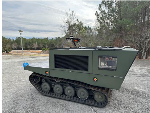
Figure 5: A custom designed and fabricated off-road tracked vehicle developed through by the Deep Orange team in collaboration with the VIPR-GS Center at Clemson University.
